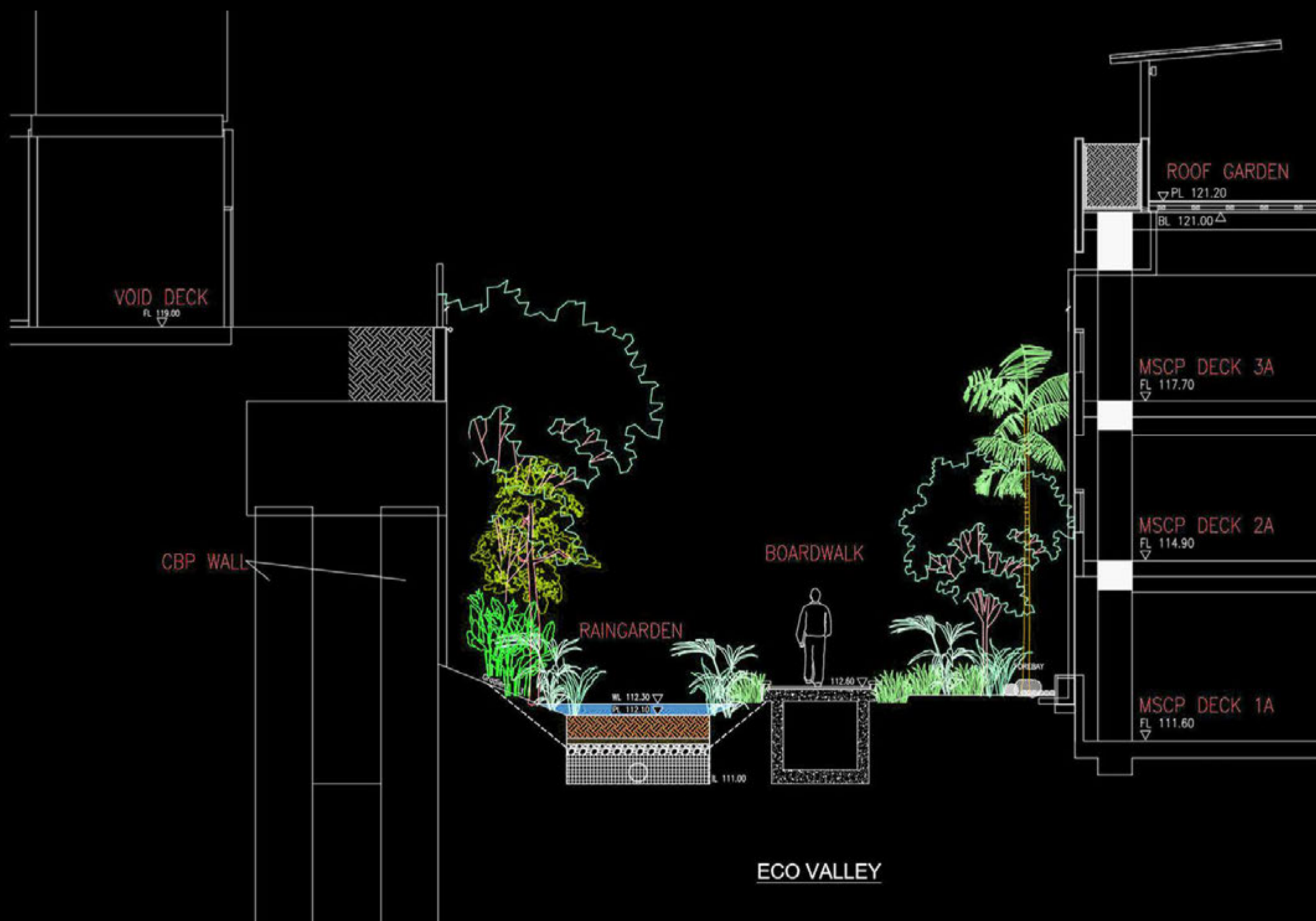
Contiguous Bored Pile wall between residential towers and MSCP
